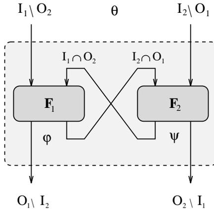
Figure 2.2: Point-to-Point communication
